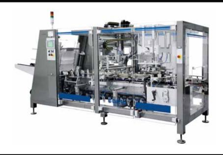
The Cama innovative solutions for RRP (Retail-Ready Packaging) provide a wide range of successful machines developed over the years. The Cama FW and IN electronic case packers are capable of packing a variety of products into RSC cases, one-piece wrap-around or two-piece display cases for retail-ready packaging solutions.
