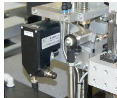
Servo motors adjust all components simultaneously
